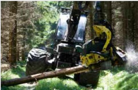
Saw Chain for use on special machines in mechanical wood harvesting and firewood preparation, robust and durable. Reduced tensions result in low levels of crack formation with low wear and a particularly long service life. Must not be used on hand-guided Chainsaws.
