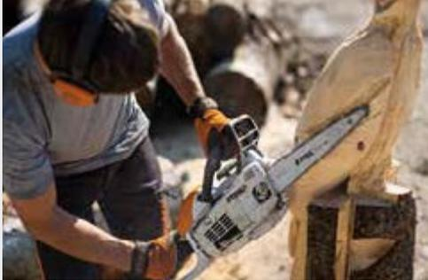
Special Saw Chain for wood carvers. Minimum vibration, very good cutting performance, shortened cutter top plate means it is not necessary to apply pressure when piercing, capable of a noticeably better piercing speed compared to conventional 1/4" Saw Chains.
